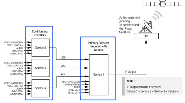
Figure 3.4: Block Diagram – One Stage of Remultiplexing
